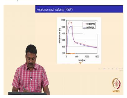
You see the time. Okay, so it is hardly 400 ms, is not it, so the metal is heated up to a temperature at the center SIS 1800°C, 2000 Calvin, let imagine metal is heated up from say a room temperature 2000 Calvin in 100 ms, it is extremely fast heating as well as the cooling rate. Okay, so within no time at battle is cool from a melting point to room temperature. Okay, so the heating rate and cooling rate can be SIS 1000 to 2000 Calvin per sec, in this case even 4000 Calvin per sec.
