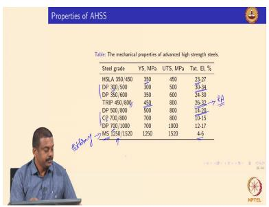
So, this table shows about the properties of advanced high strength steel's comparing with HSLA steels and if you look at it here the mechanical properties are varying from SI theorem ma Pascal until to 700 to even up to 1000 ma Pascal okay whereas in HSLA steels it is very difficult to change the mechanical properties because the microstructure is more or less fixed and the alloying elements are fixed.
