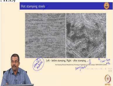
And the third generation a third significant improvement in terms of strength we achieved in automotive steels is by martensitic microstructure. So, in this process of forming martensitic microstructure we want significant change in alloying elements compared to say for example DP and trip steel. And hot stamping steel's are martensitic steels they have a similar alloying elements except some special alloying elements which increases which increase the hardenability significantly.
