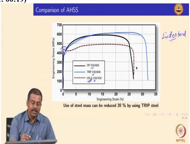
So, apart from the HSLA steels you look at it you are here so only the bake hardening Steel's would also show the Lodusband formation because the carbon is still intertial positions. So, bake hardening steel also show the yield point phenomena but IF steel do not show yield point phenomena Lodusband formation that is why the IF steel's are very attractive to; in those days to make a deep-drawn components because IF steels does not have any carbon in the intertial position.
