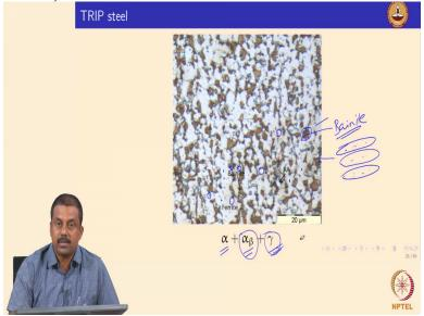
If for example trip steel again trip steel also as I explained has a very good strength as well as ductility which is slightly higher than even dual phase steel and because of this microstructure I show you now in this slide. The trip steel microstructure typically contains the ferrite and the bainite and some amount of austenite okay. So, this austenite is known as retained austenite generally we all know that austenite is high temperature phase in an iron carbon system.
