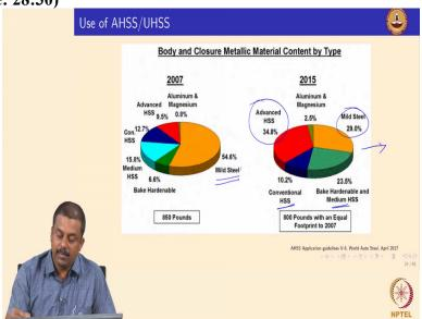
And this slide actually shows again the comparison between the various materials used in in auto two bodies so comparing 2007 and 2015 if you look at it as I actually explain the ferritic pearlitic steel's the mild steels occupied the majority of auto bodies about 55% as I showed so yeah so compared to 2017 if you look at 2015 the majority of mild steel's are replaced with advanced high strength steels mainly Arsenal phase and Trip or complex phase micro structures.
