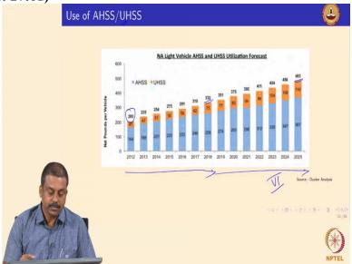
So, this graph shows the use of advanced high strength steel's and ultra high strength steel's again ultra high strength steels is nothing but an steel generally contains UTS of more than one Giga Pascal and this is the trend of usage of advanced high strength in auto bodies. So, this is in y axis we seen it pounds per vehicle and over the years if you look at and 2012 and the total amount of weight of steel that is actually advanced high strength steels used is about 205.
