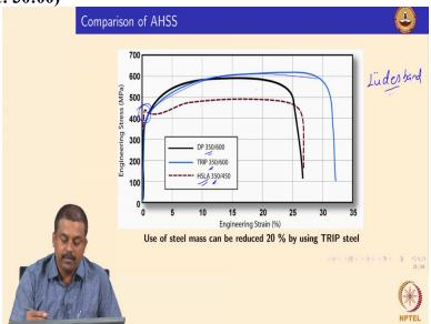
So, we will go in detail about the mechanical properties of micro structure of these steel's. So, why again the trip on DP Steel's of first generation they were very attractive in terms of mechanical properties is shown in this slide. So, this is a simple tensile testing result of HSLA and Trip and DP Steel's HSLA is high strength low light steel. So, if you look at Steel's all these three Trip and DP and HSLA the yield strength is similar right.
