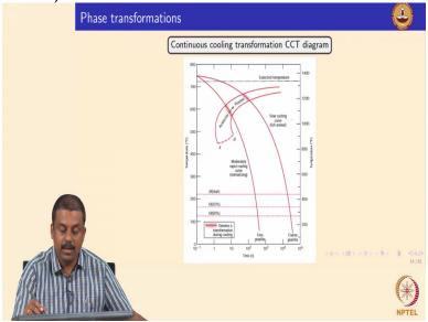
So now we will have to go back to the continuous cooling transformation diagram I already explain the first the top right corner of this CCT diagram which is explaining formation of protectoid ferrite and subsequently the austenite to pearlite transformation. Now suppose if you
