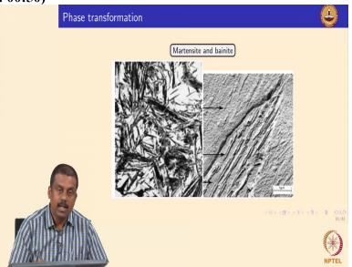
By completely diffusion-less manner so when you are rapidly quenching from austenite from high temperature to room temperature there is not you are not giving enough time to carbon to migrate triggering in the transformations. But the austenite it has to transform to another low energy state phase. So, instead of transforming and trusting and FCC structure the austenite is transforming into another structure which is body centre tetra angle structure.
