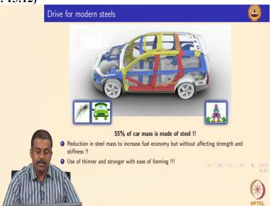
So, that drive our objective for producing Modern Automotive Steels and if you look at any automotive vehicle if you look at it in a passenger car segment as I show in this slide about 55% of the car mass are made up of Steel so obviously if someone wants to reduce the weight of the car first thing they look at is reduce the mass of steel that is used in an automotive. Show the
