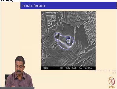
And you see in a various morphologies based on the temperature also forming so you have an invariably at the middle you have oxides of silicon and aluminum and then an epitaxial enrichment of the other inclusions that are formed in and around the oxygen inclusions.
