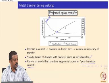
So, this graph already showed, it shows the influence of the welding current, on the droplet diameter as well as a droplet frequency. It is for a given current, you can see that and now in the A drop volume is nothing but a diameter you can say, as function of diameter and the other graph B is the transfer characteristic or transfer frequency. So, obviously a slide explains to know at the
