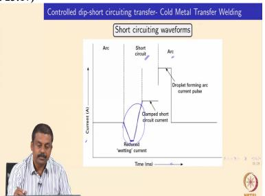
See other developments we have done in control in the heat input especially in order to minimize the damage in terms of the materials to minimize the heat input. And therefore we can also improve the mechanical properties of the weld by controlling the microstructure. So one of the developments recent days which is actually coming up in a very widely in automotive industries is the control the dip short circuiting transfer cold metal transfer welding processes.
