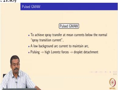
But again compared to the conventional welding process so pulsed GMAW's we use it to achieve the spray transfer as mean currents much below than the normal spray transition when you use the constant current. So, we maintain a low background sometimes to strikes to keep the arc all the time on because if you the background current reduce it to much lower than your arc may be extinguished.
