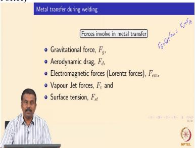
So, there are 5 forces that dictate the transfer characteristics. The first one is a gravitational forces and the gravity when you are doing in a down hand welding that the welding is done when it is then down hand. The gravity always aids interplay detachment because gravity pulls the droplet towards your work piece. And then, the, the plasma drag forces or economic drag forces
