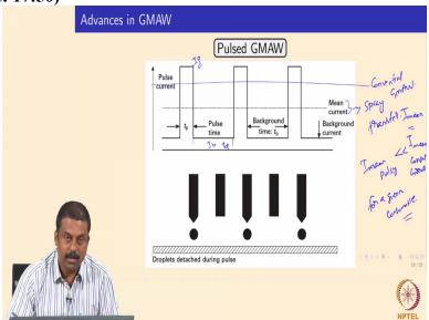
Now first I said explained the pulse GMAW the pulse GMAW process is very widely used in order to reduce the mean current of the process so that we can also reduce the and the heat input. So, the main advantage of using pulse GMAW as already explained, so we can attain the spray transition at much more mean current lower than the, if you use a constant current.
