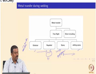
So, based on the force balance I said it explained which force is actually promoting the droplet transfer and we can classify the transfer in majority in four mode. So if you look at a free flight transfer, the free flight means droplet is transferred, transferring from the tip to the work piece in a smooth, without any contact between the tip and the work piece. So, in the free flight mode and so there are 4 types of transfer generally observed: The globular, rippled, spray and jetting spray.
