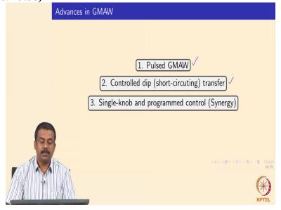
So, far we looked at the conventional GMAW process. But there are some disadvantages of using a conventional GMAW process. For example, if you use an a constant current often a given amperage like in previous graph we showed 200 amperes is the mean current already the transition current but we apply a constant amperage of 200 amperes so then you may also increase the heat input significantly okay.
