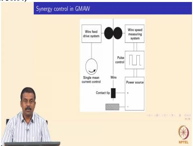
So, these kind of the complex mechanism, complex process parameters variations can only be controlled nowadays by the invention of synergy power sources, where the because of the control over the input current and the voltage as well as the wire feed rate and using a micro processes based on the power sources so we can independently control the wire feed systems, the current voltage, we can measure the waveform simultaneously.
