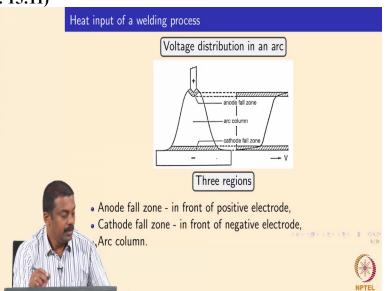
So generally the np can be calculated for a given composition of the filler wire and the configuration of the process. Generally the NP is calculated based on the polarity for example if you look at typical GMAW setup. So, we have three regions in the and the GMAW a schematic if you look at it and if your electrode is positive and you have an anode which is your filler wire and you create an anode fault zone and an arc column, surrounding the anode.
