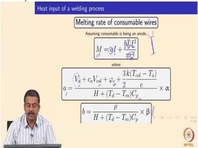
So, the other important parameter in consumable welding process is the melting rate of consumable. So, that is also very important to understand because that determines your well built geometry and your productivity. So, that is again is a function of the amount of heat that is transferred to the electrode whether it we are going to keep the electrode as a positive or negative. So, in this case, so if your electrode is anode.
