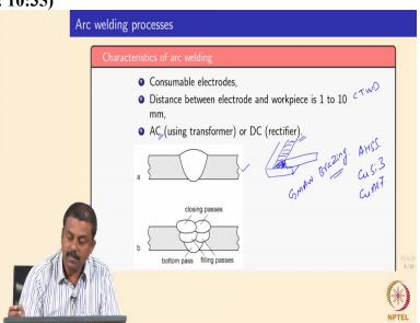
And if you look at the actual characteristic of the arc welding process so we use the consumer electrodes. Generally the distance between the electrode workpiece it is also known as CT WD. So it is contact ripped workplace distance. So contact tip is the electrode container which actually transfers the electrode towards the work piece. And the distance between the contact tip between and the work piece is very critical because that is going to determine the stick out length.
