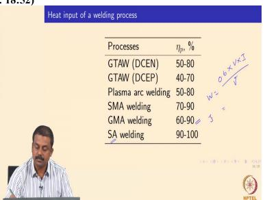
So, that is why generally in gas tungsten arc welding process the efficiency is quite low whereas in a GMAW welding process you can have the efficiency of the process going up to 60 to 90 %. And based on the heat transfer from the arc to the work piece and you also see I listed a various processes the other variant of GMAW is the submerged arc welding process which has an highest efficiency why because the arc envelop is completely covered by the flux in a submerged arc welding process.
