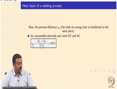
So then, the efficiency can be calculated very easily. This is the process efficiency is nothing but the total arc energy that is transferred the work piece right. So in this consumer electronics classes so you also melt the consumable and then transfer the droplet to the work piece so the total efficiency is the amount of heat generated in the cathode as well cathode fault zone plus the heat generated in the anode fault zone.
