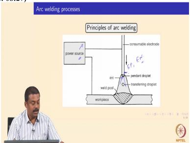
The other aspects of GMAW which you have to see, so again the schematic is shown in this slide, so this can be seen to understand the entire the transfer characteristics and the cross-section of the weld pool what you generate. So, we have the consumer electrode and the electrode and the work piece is connected to a power source. And these power source transfers the current it can be either alternating current or direct current.
