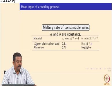
So, I have given some of the constants a and b, it is used for commonly common welding wires. For example, if you have a 1.2 millimeter a plain carbon steel as a filler. So, we can get an a and b calculated from the experiments. It is say or example, your, a vary from 0.3 and then b is 5 \*10 power -5 and using this value if you know the stick out length the L as well as your welding current and your radius in this case diameter is 1.2 mm in diameter.
