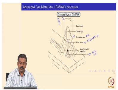
So we will move on to the GMAW process gas burn arc welding process and most of you familiar with the schematic of GMAW. See this is one of the oldest processes availing processes developed to weld conventional materials. So there are three important parts, you can see here. Now, the first important foremost important is the shielding gas and shielding gas is also known as arching gas because we strike an arc using this shielding gas and the filler wire.
