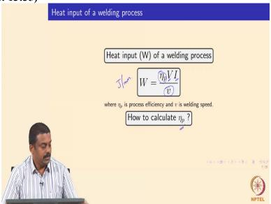
So, in this GMAW, the heat input is determined by a very simple equation. So, where we have the voltage and current which is actually passed to the, the current is passed to the system voltage V. So, the heat input which is calculated in joules per mm which is not is actually nothing but the np which is the process efficiency. Process efficiency determines how much heat which is generated in arc transferred to the work piece times the voltage of the circuit.
