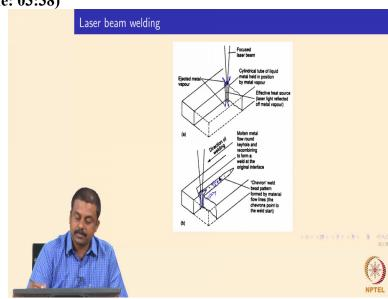
And if you look at in depth now what is happening inside the key hole, so basically you form a key hole by the evaporation of the substrate and once you have evaporation you eject the metal vapour that is formed in from the top and bottom of the key hole. And because of this evaporation you also have various forces that are generated and we will see in the subsequent slides the forces and how we can balance it to from the stable keyhole.
