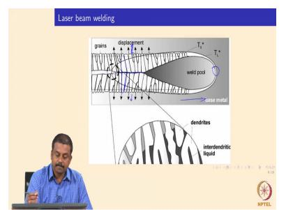
So, as shown in this diagram, so, what we looked at in the high speed video, this is actually also shown in this schematics. So we have a weld pool, a keyhole is somewhere over there, here, is formed. So if you link it with the keyhole so we have a liquid pool that formed in a tear shaped manner when the source is moving along this direction the weld pool solidifies under this process. So, we have a solidification that is happening from the fusion boundary towards the weld center line.
