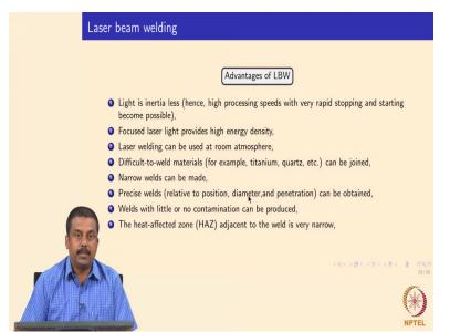
So, we move on the advantages of laser beam welding. The main advantage here is, laser is extremely manipulative. So, we can transport laser from one location other locations and it can also be turned and off very rapidly. And also laser is inertia less. So, then, due to that we can process it much more rapidly and transport it one place to other place very easily. So, if you focus a laser light into a substrate, we can transport the energy almost without any loose, without any loss in energy.
