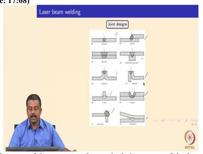
So, joint designs because of the very easy the manipulative nature of the laser and laser can be focused into various joints, so we can make a bud joint and lap joint. You can also make a spot weld using laser which is also considered advantageous in various aspects so in a spike and then a flange or even in edge joint and a T joint and a plug joint in this case. That is similar to what you do it in the conduction joint I can be do it in a corner weld or in a Zinc weld.
