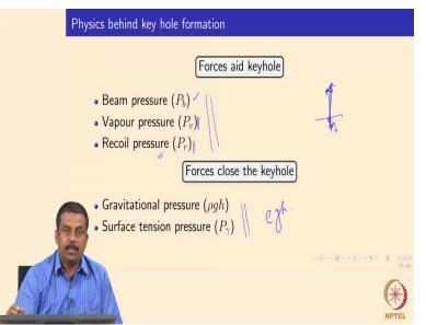
So, some physics about keyhole formation and then we wind up the laser welding. So there are 5 important forces that control the Keyhole formation, as I had already explained about keyhole formation is extremely critical in laser beam welding. A good stable key hole is formed by balancing the 5 natural forces and during welding. So there are 3 forces which actually aids the keyhole formation and two they try to close the key hole.
