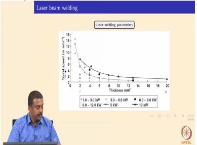
So, the laser welding parameters again it is also function of thickness and the travel speed. And if you use a larger thickness material for example 12mm material so, you can choose laser power
