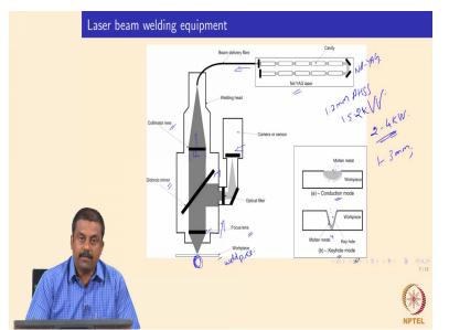
So, the once we have a laser source obviously we need to make a welding setup. So, this slide shows a typical welding setup, used in one of my earlier laboratories in Netherlands. So, we had an Nd-YAG laser okay so, the Nd-YAG laser medium it is schematically shown over here. So we have one so about 10 gain mediums made of Nd-YAG material and we generate lasers and this laser is actually sent to beam delivery cable towards an welding station.
