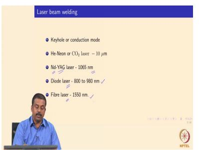
So, if you look at the various lasers and that are commercially available as I already explained you know, based on your intensity and the focal point we can either do a welding in keyhole mode or full presentation mode or in conduction mode. Some other applications of lasers suppose if you want just do in a surface hardening treatment, you want to deposit powder, using a laser source so, in that case, know, we limit the damage to the microstructure or the substrate to minimal levels.
