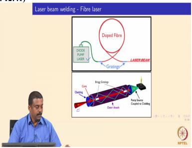
So apart from Nd-YAG lasers, the recent development in to in laser industry is the fiber laser. So in fiber laser, so we do not have an solid gain medium. And instead of a gain medium we have glass fibers which actually acts as an gain medium. So in this case the excitation or the pumping is done using on a laser itself. So we generate a laser using a diode source and then this laser at
