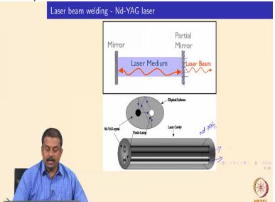
And which is actually used in various applications. So one of the lasers I am going to talk about today is the Nd-YAG laser. Nd-YAG laser as I already explained is so the gain medium the neodymium yttrium aluminum garnet is actually used to excite and used as a gain medium. That means that you know the when you have a pump electron which is sent to the gain medium and you excite the electrons of the gain medium and when these electrons return to ground state they release laser photons.
