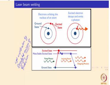
So, some fundamentals about lasers so this you already have familiar with the yeah you already have familiarity with these diagrams. Basically how do you generate laser before going to that we will also understand what is laser signify laser is, so light amplification by stimulated emission of radiation. Each word has its very significant meaning. So in this case, the stimulated emission, so what, and what does it mean here?
