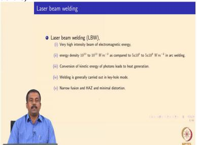
So, laser beam welding as I told we use the laser as a heat source to heat up the work piece and melt and then form a fusion joint. So the laser we all know that it's a very high intensity beam of electromagnetic energy, so we make use of the electromagnetic energy the photons the light photons to heat up the work piece. And how do we heat up the work piece? Because when you
