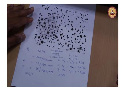
Now, let us start measuring this the P P first. So, what I am doing is I am placing this probe on the microstructure in a random orientation. So, let us not put like this try to keep a symmetric it should be random like this. So, I am just putting it like this so, what is that first I have to do, I have to just count the number of grid points. So, 1 2 3 4 5 6, 1 2 3 4 5 6 so, about 36 grid points I have so, capital N is equal to 36.
