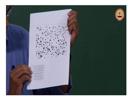
So, and we are going to use a probe of this nature which is of about a grid of this, so, now what I will do is, I will now demonstrate using this probe how are we going to calculate the point fraction and then how that is related to area of fraction that is P P and then again the second demonstration professor mentioned about how to measure the P L, that is which can be related to the average diameter of the particles of this microstructures.
