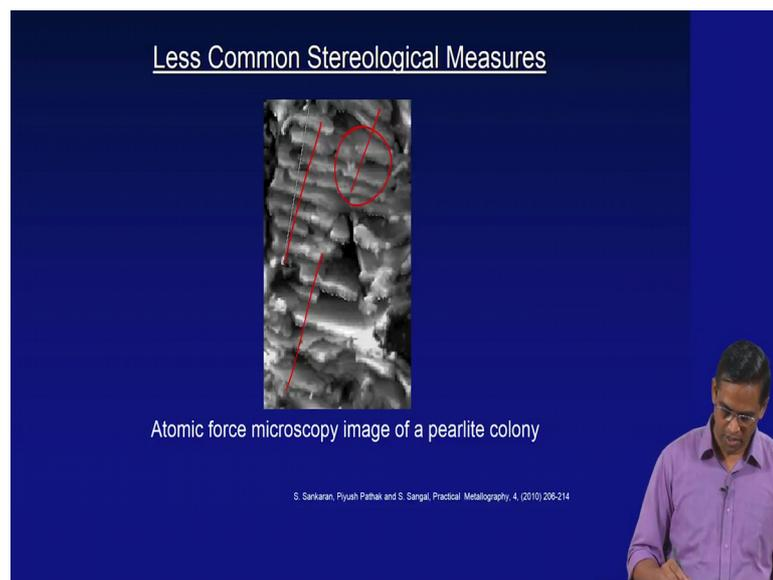
And if you look at this microstructure the, this is an again and a atomic force microscopy, image of a pearlitic colony where you can clearly see that the cementite plates platelet us all; just is a stack of plates in between the ferrite region. So, what we are interested is actually the spacing between these two or the set of cementite plates.
