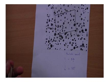
You can keep this graphite nodule, nodular microstructure like this and then the probe can be kept like this and you can just keep this and then start counting. So, the rule is, you have to exclude this particles which is intersecting these lines and include the particles which is intersected by this line.
