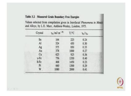
This is one plot which I had, this is one table which I have included because this table gives the relationship between the grain boundary energy and the surface energy. That is between the solid and the vapour surface. Generally, it is seen that this ratio of grain boundary energy to a surface energy transfer to be close to around 0.3.
