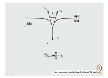
Then depending upon the angle which it makes with respect to if we drop this angle theta is you know then we can calculate. This expression could be derived. These essentially that balance of equation which we have written. 1 2 and 3 this boundary and then we can find out that grain boundary energy depends upon twice gamma s v 2 cos theta by 2. This way we can find out the energy of the various types of boundaries could build it. These are all experimental determination of grain boundary energy.
