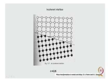
So, in an incoherent interface what happens is that no strain is being accommodated right. Up to the end up that interface the perfect lattice matching is being maintained on either side of the crystal, whatever the lattice parameter, which is there here the same thing we will be seeing right up to the interface. Because there is in the case of coherent is strain there is a lattice parameter is changing because they wanted to maintain the continuity across the interface correct.
