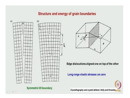
So, essentially suppose we take a crystal. They are single crystal and another identical one, we take it with the same orientation it is placed and if they are joined together. This can give rise to another one single crystal.
