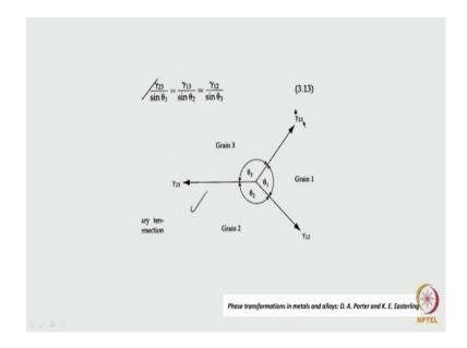
So, this is the between grain 1 and grain 3, this is the grain boundary energy between 2 and 3 this is the grain boundary energy gamma 2 3 here, gamma 1 2. If that is the case the angle between this boundary this easy to derive, and only just giving that formula, that is the gamma 2 3, divided by this sin theta 1, 3 divided by the opposite angle gamma one 2 divided by obtuse angle, which is sin theta 3. This have to be equal. That is because it is an energy balance which has to be done.
