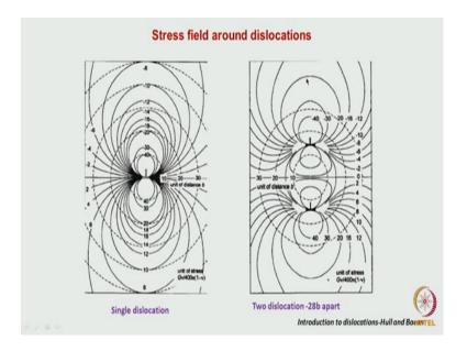
If a single dislocation is there this is the way, the stresses it is iso controls of the stresses are being or shown both tensile as well as the compressive stresses.
