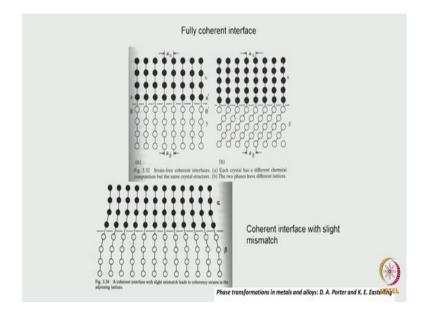
So far what we considered was essentially with respect to a single phase right, that small angle boundary and high angle boundary and special boundaries. These are all the type of boundary and depending upon the energy between the various types of boundaries what is the angle which will make between the boundaries. Other type of a boundary which we have to consider is essentially is when we have precipitates are there which has a different composition compared to that of the matrix.
