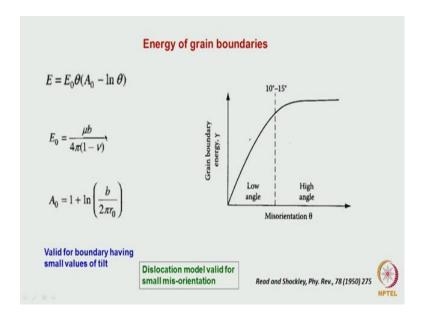
Essence of it, essentially is that this is e 0, which is essentially depends upon the material properties. We are it is assumed that it is a material having a modulus mu, an infinites material and Poisson's ratio nu. And r 0, is the core of the dislocation. This is the way the energy is varying that final formula which we get it; that means, that as theta increases the energy of the boundary also increases.
