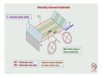
That is what essentially is being shown here. This is the x direction which is the habit plane, this is the y direction this is a martensite which has formed and it set invariant. So, I am calling in MT 1 at MT 2. This is with respect to a parent; this is how that tilt which has come. If you look at MT 1 with respect to a original parent lattice this is we are
