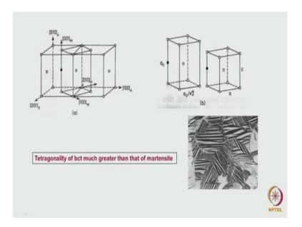
Now, that is exactly what is it being shown. And typically when this sort of martensite is a plate martensite which comes which is essentially a twin related structure. As I mentioned that why twinning is required this twinning is the one, which is responsible for compensating further to make strain in one direction 0.
