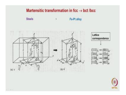
Let us look at the martensitic transformation. Iron at high temperatures about 900 degree centigrade is in fcc this transform to bcc ok below 910 I think to bcc structure martensite degree. Most of the time that iron contains carbon, so since the carbon is within that sample, it is not able to come back to the bcc structure, the carbon got stuck at different positions that transforms that changes the unit cells along whichever direction that
