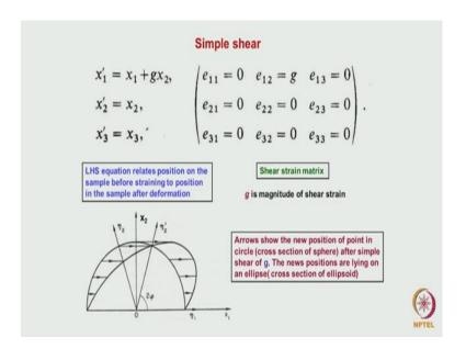
The crystallographic theory we will look it. Before we go further let us recap that because we are talking about this transformation and as I mentioned, So, many times homogeneous shear which is taking place in this material, let us look at the characteristics of a homogeneous shear before we go into the martensitic transformation theory.
