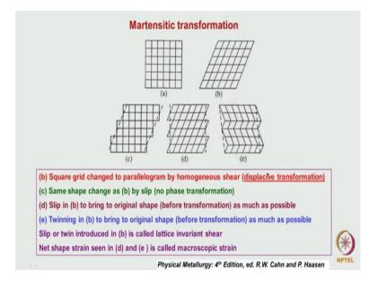
So, this is essentially what I had shown in this transmission. So, here what has been done is that that inside, the square a 2 dimensional small lattice is also being shown. The
