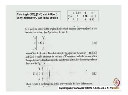
And another is that, we have studied earlier that when we have given such strain and deformed from one lattice to another lattice. We can using the lattice correspondence we can find out the directions and planes corresponding to the same direction in each of the lattices. That is what essentially the matrix corresponding that is given what is the strain matrix here. The strain matrix now it turns out to be in terms of the BCC these 0.1000 this is,
