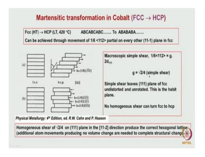
Let us consider some specific case. One martensitic transformation in cobalt let us consider. This cobalt is at high temperature it is hexagonal close packed. It transforms to face centered the closed packed, that the face centered cubic lattice at lower temperatures below 420 degrees centigrade. So, above 420 degrees centigrade it transforms to HCP. What is the stacking sequence in these lattices? It is essentially A B C A B C is the stacking sequence in HCP.
