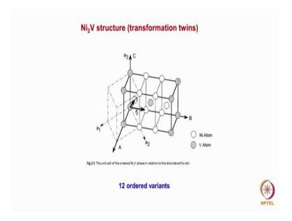
This is another structure, but we will not go into all these structures, I can show examples where a twinning occurs in ordered a structure. Especially in ordered structures we can have 2 terminologies which we use one is called as 2 twin where the ordering of the disorder the ordering of the lattice is being retained after twinning in the twin lattice also, another is called a pseudo twinning where the ordering is not being maintained.
