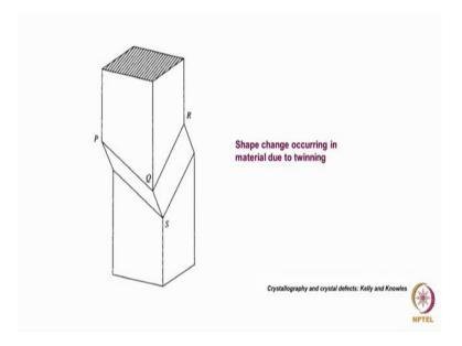
Mechanical twin essentially if you try to look at it whenever a twinning occurs as we can observe there is a deformation could be seen externally and the sample surface and we can observe that this is a homogeneous tilt of the external surface which is occurring.
