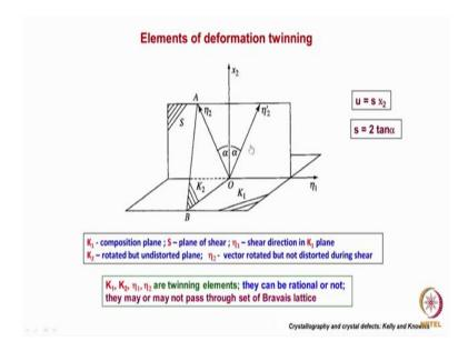
When we considered twins as a general phenomena of homogeneous deformation we understood that there are 2 planes are there, there is 1 plane which is called as a K 1 plane or a composition plane which is undistorted and unprotected. And there is another plane which is a undistorted, but it rotates during the shear homogeneous shear transformation.
