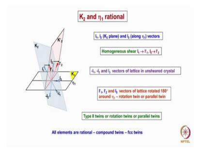
Now, let us consider the case K 2 and eta 1 are rational here what I had shown is the projection of the various planes, this is K 1 plane, eta 1 is the shear direction in the K 1 plane, assume that the; and 1 1 and 1 2 are 2 vectors like the way we considered earlier when K 2 is a rational thing we can find some 2 unit vectors in the K 1 and K 2 plane smaller, not even to small vector lattice translation vectors. These 2 vectors may
