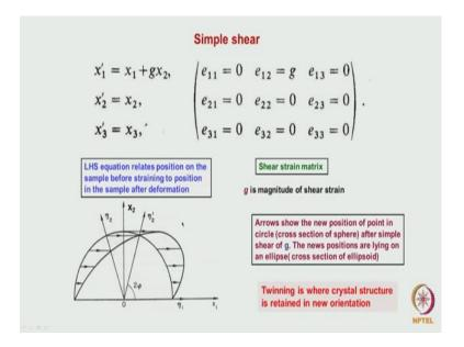
Let us just look at a simple shear. In a simple shear what we do is only that if you look at the strain tensor, which is being given, it is only one direction we are giving and simple shear. What is being shown here is that we assume that the original shape of that sample we assume it to be hemisphere. This hemisphere when we apply this shear, what we are applying it is called as a simple shear.
