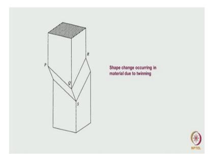
Before we do that if you look at a material, how does it look like when a deform it. If a material deforms by twin are assume that a material is deforming by slip. Suppose, this is the shape of the sample, lot of dislocations have passed through the sample, various this made of form and there pass through it. Then the material would look like this way, externally we can see this correct this is how with that stuff it happens. How this can be verified whether it is occurring or not is that.
