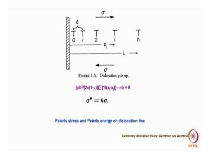
Here what we have done is that, when dislocations of these types have generated. This is the sort of here suppose this there is a boundary which is going to be there. Assume this a grain boundary. So, when these dislocations reach this grain boundary look at the grain boundary will stop that. That means, that in the same slip plane there are dislocations one after the other behind one another dislocation like this is there.
