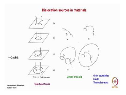
Here, what is being assumed is that a dislocation line is there; a segment of the dislocation line that is the B C is in the slip plane. And A B and C d/ are out of the slip plane. If we apply s burgers vector is in this direction, if you apply a stress what is it going to this is being pinned, under the action of the stress the dislocation will climb we would like to bend correct.
