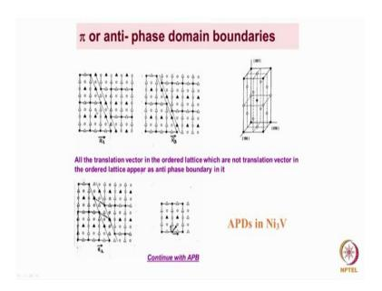
And showing that this same crystal structure. This we considered in an ordered lattice if dislocations are present, what is the type of dislocations could be there super dislocations. And the same structure like if you remember how we define that a p b in a 2 dimensional lattice. This is also this precipitate forms in many cases like nickel 3 vanadium.
