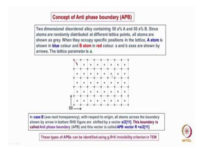
If you consider the best example is to take a 2 dimensional lattice. The lattice which is being shown here is essentially a disordered lattice actually it is an alloy you consider to be alloy which contains of an atom A and B which is in 50 percentages A and 50 percentage B and the atoms are randomly distributed.
