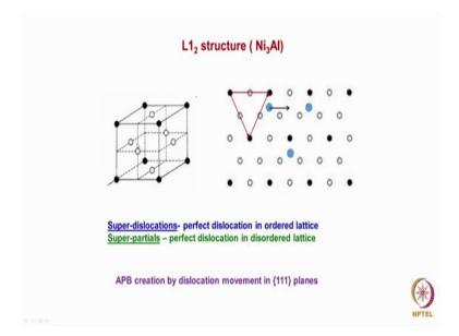
Here, if you look at it, the aluminum occupies that corner positions nickel are the phase centers. This is the close packed plane here also is 1 1 1 plane. In this plane if you look what is the perfect translation vector it is from going from here to here, or from here to here or from here to here. In the disordered lattice if you consider half of it from here to here is essentially what is going to be the translation vector in the disordered lattice.
