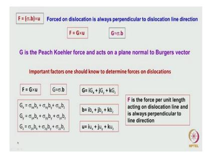
This one sigma that b because here we started with; with respect to a plane normal the force which is acting with respect to a plane normal and now using this mathematics we had come to this one where this is a forces this equivalent to because b is a vector correct. So, the force which is acting across a plane which is perpendicular to the burgers vector this force is called as pitch coiler force is this clear.
