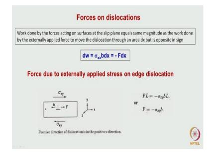
The burgers vector is in the negative direction then sigma x y, we supplied in this direction and with respect to a definition which has been used if we substitute for the value of b here the b is minus because in the negative direction the force turns out to be in the positive direction this way we already we can find out the situation becomes more complicated when we look at a force on a screw dislocation.
