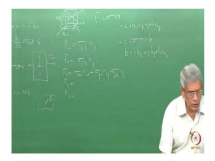
Then this is how we defined x, y, z, with respect to this coordinate system which we have chosen on this face will have sigma xx, in this direction sigma x z, correct, this is how the similarly on all the other faces are there if we have these components which have known what will be the force which is acting on any random plane that expression which we have derived.
