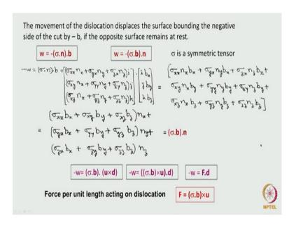
But what we have to look at this now is that when this force is being applied suppose it makes that dislocation move because d is the movement of the that dislocation a unit vector in the direction of motion of the dislocation when at dislocation moves what is going to be the work which is going to be done is this force times the burgers vector dot
