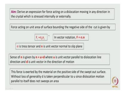
That is what we will look at it, there is we wanted to find out the force which is acting on a dislocation which is moving in any direction in the crystal which is stress internally or externally.
