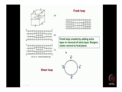
Then another type of a dislocation which we considered are the frank dislocation or the frank loop. This essentially is that if we remove one of the layers partly not completely like.
