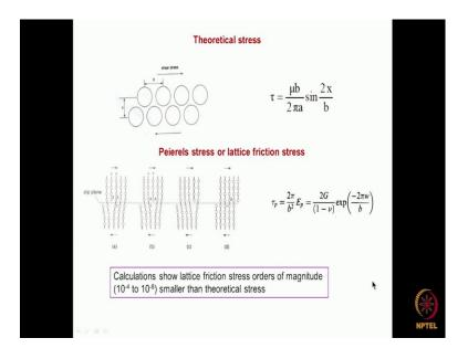
To understand this better, I had given a comparison between the theoretical stress which is required for deforming a material in the absence of a dislocation and one when deforming the same material when dislocations are present. As we have mentioned earlier in the case of a material there no dislocation is present like an example the viscous where only point defects are there no dislocations are there, and one layer of an atom.
