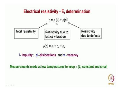
Another technique which also can be used to get information about that defect concentration is electrical resistivity or conductivity measurements. Especially in metallic sample electrical resistivity has been used to get information about point defect concentration as well as the migration energy; not the point defect concentration formation energy as well as the migration energy of defects we could get that information.
