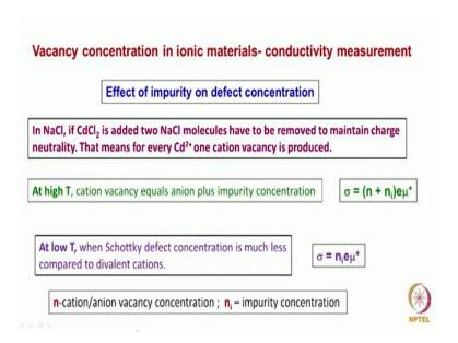
That is essentially it will be not formation plus the mobility, because the rate at which it is moves is not like that of an electron. So, the mobility information also comes into the picture. This will become clear when we go along. If you look at that impurity concentration, because no material is pure material some impurity will be present the impurity in most of this ionic material could be. Another ion which has been added which has got a different balanced stage.
