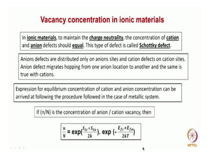
Though so far what we talked about is vacancy concentration in essentially metals. Suppose we consider vacancy concentration ionic materials: the material. The resistivity in ionic material or the conductivity in ionic material does not depend upon the electron concentration all depends upon the charge carriers which have the ions which has to move. And that is what is going to control the concentration. And another important fact
