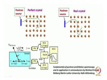
Suppose a defect is there; the region where the defect is present like here in this case if you see it. When there is no defect irrespective of whichever be the site it moves and reaches, it does not matter whether this point or this point it is going to take almost an identical delay time which is going to be there, because the density of electron is going to be the same almost in all the regions.
