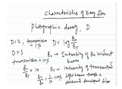
One of the most important properties of x-ray films is what is known as photographic density which is written as d and D is given by this expression log (B0/BT) wherein B0 is the intensity of the incident x-rays of the intensity of the incident beam and BT refers to the intensity of transmitted light through a completely darkened and developed film so you take the film which is already developed and darkened and then measure the intensity of light which is passing through it.
