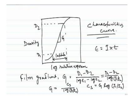
And if you now plot this identity with the exposure or log of exposure then you get a curve like this okay so this curve is known as the characteristic curve and every film is supplied with this particular curve the manufacturer has to you know do the tests and provide this curve for a particular film and from this film you can derive certain other properties for the film which are important for forming the image on a radiographic film.
