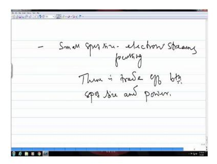
But remember one thing when you have a small spot size you have electron streams focusing on a very small area and this will lead to intensity locally around that area and as a result of that you know you have to control the power you have to reduce the power so that there is no excessive heating on the target so therefore when you try and use small spot size there is always a trade-off between the spot size and the power okay.
