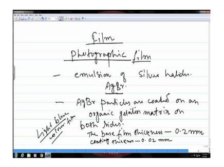
And the second one is the film on which you capture the image okay this is primarily a photographic film which interacts with electromagnetic radiation like visible light or x-ray radiation and when it interacts it darkens as I would have said you before also in the beginning when I showed you that radio graphic image of our hand so there also you saw that the whole plate is darkened and only the image of the hand you can see some white contrast for the bones okay.
