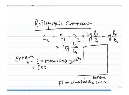
So when you see a contrast on the film it essentially means that between two regions that you see a contrast they have different density d okay, so the contrast or the radiography contrast is nothing but the difference in the densities between two regions so this is the second property of the film which is the radiographic contrast so as I said this is nothing but the difference in the densities between two regions if we call this as CS this is the density difference okay.
