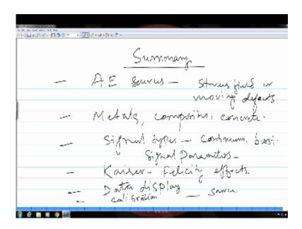
So with this we come to the end of this particular topic so let us take a moment to summarize before we close up so first we learned about the sources of acoustic emissions and then we saw it is due to a stress field or moving defects which generate some kind of elastic wave inside the material that is how these emission waves are generated okay and then we talked about the sources with respect to different kind of material and systems like in metals composites and concrete.
