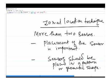
And if you want to get some idea about the location of the sources then you have to use the zonal location scheme so in the zonal location technique you have more than two sensors which are placed at different locations on the structure which is being examined and in this case the placement of the sensors is critical because where you place the sensor at that particular location you should have a potential source of acoustic emission around it.
