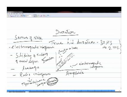
Now the important aspect about acoustic emission testing or for that matter for any other entity testing is to filter out the noise okay because we have seen in these case especially that there
