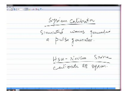
So as you would have seen before in order to calibrate a system you need to have some reference which could generate a signal which can be used as a defect signal and calibrate the instrument okay so in this case also you need to simulate acoustic waves which come out from defects okay so you have to use a pulse generator which can simulate acoustic emission which comes out from actual msn events we can use simulated waves generated by a pulse generator.
