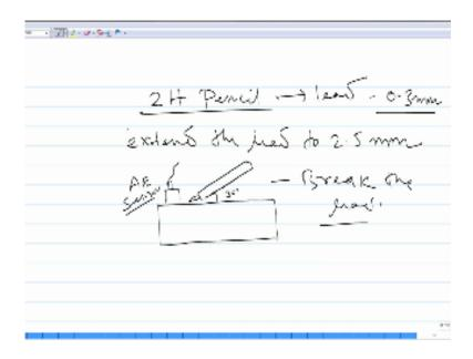
So what is done in this case all you need is a 2h pencil and you simply have to break it okay you have to simply break the lead of the pencil and due to that fracture event okay you could generate lot of acoustic emission so as I told it will be like a phenomena like a damaged phenomena which is similar to the damage and effects that you can expect inside components okay so you take this pencil and then extend the lead up to about 3 mm2.5 mm or 3 mm and this pencil lead is
