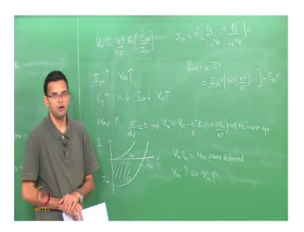
So, We have written down the expression for the open circuit voltage,  $V_{oc}$  approximately  $\frac{kT}{e} \ln \left( \frac{I_{ph}}{I_{so}} \right)$ ;  $I_{ph}$  is your photocurrent which depends upon the intensity of the light and  $I_{so}$  is your reverse saturation current, which depends upon the intrinsic career concentration  $n_i^2$  and also on the diffusion coefficients, diffusion lengths and the concentration of p and the n regions there is a term e here.
