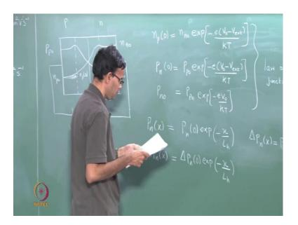
So, here is my p-n junction. This is my interface, these are the depletion regions, this is p and that is n. We have a p-n junction in forward bias, so p is connected to the positive and n is connected to the negative. We saw in this case that we can plot the concentration of holes, so that there is some excess holes can do the same with electrons. So, you have some excess electrons.
