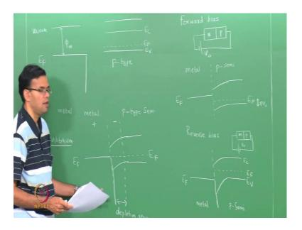
So, Once again we have the vacuum level, you have the Fermi level of the metal and this is phi m and this is the metal. We now have a p-type semiconductor. So, This is  $E_c$ , this is  $E_F$  and this is  $E_V$ . So, it is a p-type semiconductor so that the Fermi level is close to the valence band.
