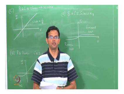
So, the I-V characteristics will just be a straight line and the slope of this line will be just 1 over R. Part-d, sketch the I-V characteristics when B is Ohmic. So, B is Ohmic and then C is Schottky.
