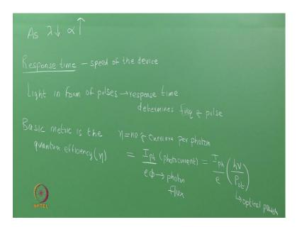
The basic metric of a Photodetector is called quantum efficiency. So, the quantum efficiency is defined as the number of carriers that are generated for per photon. So, this intern is related to the photo current divided by the flux of the photons. So, I ph is the photo current this term phi is the photon flux. Another way of writing this, set it is Iph over e and flux of the photons is depends upon the power of the incident radiation and the energy.
