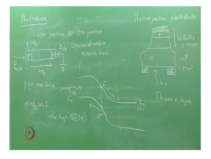
In the case of a Photo diode we use a p and then n material so that, you form a junction. So, these can be a simple p-n junction or modification of that which is a pin junction. So, electron hole pairs are generated either in the depletion region of the p-n junction or they generated in the intrinsic region. These electron and hole pairs are then separated by applying a reverse bias to the junction.
