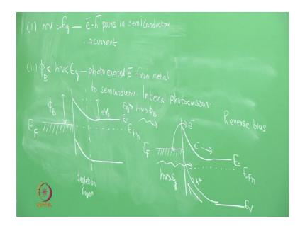
We had seen earlier that there essentially 2 kinds of metal semiconductor junctions: 1 is your Schottky junction, the other is the Ohmic junction. So, in the case of photo diode we want a depletion region so that, we can generate electron whole pairs. Now, the Schottky junction is the 1 that has a depletion region. So, we use a Schottky junction to form your photo diode.
