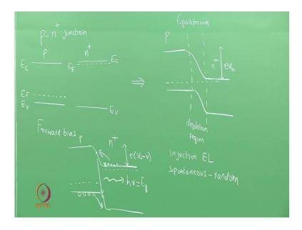
So, let me start with that first. So, consider a simple p and plus junction. The n plus means that the n region is heavily doped. So, when we form a junction the depletion region is mostly within the p side. So, I have my p side E f, E v and E c this my p side and I have my n plus
