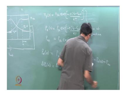
Here is my P n junction, this is my interface. These are the depletion regions is p, that is n. We have P n junction in forward bias. So, P is connected to a positive and n is connected to negative, we saw in this case that we can plot the concentration of holes. So, that there is from excess holes and do the same with electrons. So, you have some excess electrons. So, we can mark the different regions is n naught is P n naught, P naught and the extra carriers some be P n of 1 is P n P see.
