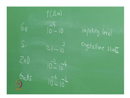
Some examples of semiconductors, Germanium, Silicon, Zinc Oxide, Gallium Arsenide, some of the typical values of resistivity: Silicon is around 0.1 to 10 to the 3; Zinc Oxide is 10 to the minus 2 minus 4 is lower; Gallium arsenide minus 6 to minus 2. In all of these cases have given arrange of values the actual resistivity, all the conductivity depends upon the impurity level and also the crystal in state, whether you have a single crystal or a polic crystal.
