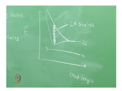
Energy verses bond length we have Lithium which is 2s 1 you have 1s inner shell, you have 2s 1. So, this is the energy band here and there are a total of 2 end states, but each Lithium atom will only contribute 1 electron.
