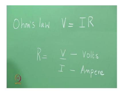
Ohms Laws states the voltage is nothing, but the current times the resistance and other way of writing it is resistance is voltage over current. A unit of a voltage is volts a unit of current is Ampere. Now, resistance depends upon the dimensions of the sample. So, if we have thinner material or if we have a wire with a smaller diameter then the resistance is higher. So, we need to think of a parameter that does not depend a part on the dimensions of the sample.
