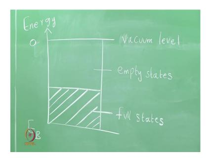
So, in this case the energy is on the y axis we reference an energy level calls 0 which is the Vacuum level. So, let me call this is the Vacuum level and this has a value 0. So, everything can be reference to the vacuum level. So, you have an energy band that is halfful. So, in this case these are all the full states and these are all the empty states. So, how do we arrive the fact that the energy band is halfful, we go back to the energy verses the bond length diagrams.
