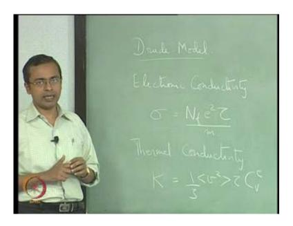
So, the Drude model, this is what we have developed over the last few classes. The basic idea behind the Drude model, is to use the ideas of ideal gases, the kinetic theory of gases and to, merely with minor changes if any, to extrapolate these exact same ideas
