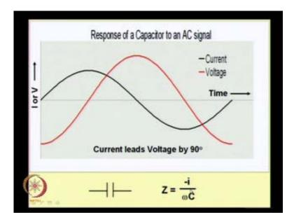
So, here for example, we have a capacitor. In a capacitor the current and the current and the voltage are not in phase, in fact current leads voltage by 90 degrees meaning when
