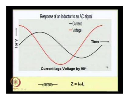
In a similar, but opposite manner so to speak we actually see that in an inductor the opposite is true. We have the current which lags behind voltage by 90 degrees. The similarity is that between a capacitor and inductor is that in both cases the impedance is entirely imaginary, there is no real component to it. Again there is also a dependence on the angular frequency omega. So, that is also present here except that now the angular frequency is there in the numerator itself.
