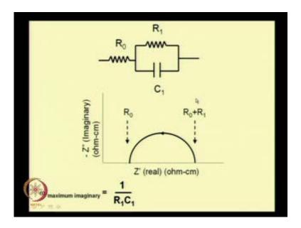
So, in a real system like I said you will have aspects of a capacitor and an inductor and a resistor all thrown in. So, what we would normally see would be a material which would have say for example, part of it behaving like a resistor which would then behave, which would then be in series with a resistor and capacitor and parallel.
