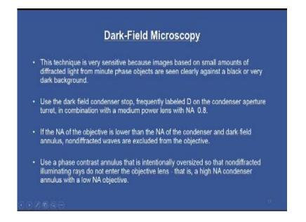
So it is a very simple design and this technique is very sensitive because image is based on small amounts of reflected light from minute phase objects are seen clearly against a black or very dark back ground. If the numerical aperture of the objective is lower than the numerical aperture of the condenser and the dark field analyst non diffracted waves are excluded from the objective. (Refer Slide Time: 02:49)
