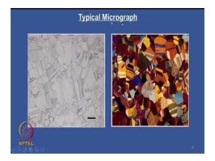
And you see that this is a typical micrograph of a polarized microscopy the material is under the examination is brass and you see that bright field elimination gives a kind of contrast a polarized light gives her extraordinary a contrast now I will take you to the lab.
