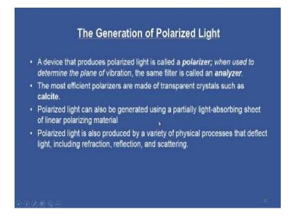
And we will see that much more details a device that produces a polarized light is called a polarizer, when used to determine the plane of vibration the same filter is called an analyzer please understand we have the same material which being called polarizer as well as analyzer when it is called polarizer when it is used to determine the plane of vibration the same filter is called an analyzer.
