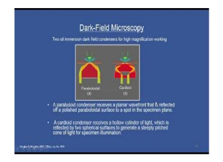
So you can have two kinds of oil immersion dark field condenser for this optical setup they are very simple in nature and you know that the principle of oil immersion objectives already we have seen that so I will skip and while quickly move on to the next variant polarization microscopy.
