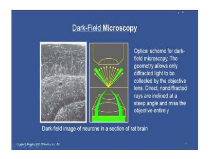
So let us look at the dark field microscopy the slide shows one typical example of the biological sample it is a dark field elimination you can see that all the features very minute features are clearly illuminated and if you look at the optical setup or the optical scheme for a dark field microscopy the geometry allows only the diffracted light to be collected by the objective and direct and non defected rays are inclined at a steep angle and miss the objective entirely.
