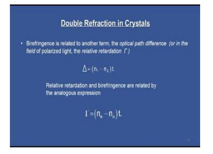
Birefringence is related to another term the optical path difference or in the field of polarized light the relative retardation so optical path difference and related retardation or the similar term but relative retardation is used in polarized light scheme otherwise it is in generally in optical literature it is reference to optical path difference which we have already seen  $\Delta = (n_1-n_2)t$  where t is the thickness of the glass or the medium.
