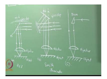
let me draw the schematic suppose this is the this is the light saying which is coming from the source so normally it is passes through a glass slit and then they are all reflected then you have the objective and then you have specimen of face this is object let as be A.
