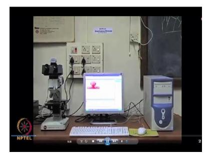
And the another one is which is the image analysis system, that also I just introduced just to recap. You can see that objective lens again system stage. So these objectives will have three or four depending upon the microscope ranging from 5x to 50x to 100x. And you can see that al the objectives are marked with their specification of their magnification, refractive index details. And depending upon our interest we can choose any one of this objectives to view the micro structure.
