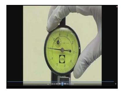
And this is a very important tool for ceramic material and in some cases people use it for metal as well but normally it is used for only ceramic because in metal you use it with the disc punch and each one is about a 10 micron division. So you have you can control the micron thickness so in order to do this cutting you put this ceramic it is typically a boron carbide and nitride or silicon carbide and then,
