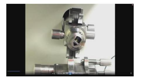
And you have the specimen stage here this is a specimen stage and you have all the gauges to control the stage movement left right and top bottom and so on. And this is the specimen holder you can open this and then put the specimen corresponding specimen inside and then lock it up into the arm. We will show the typical action of the cutting and then we will proceed with the actual demonstration.
