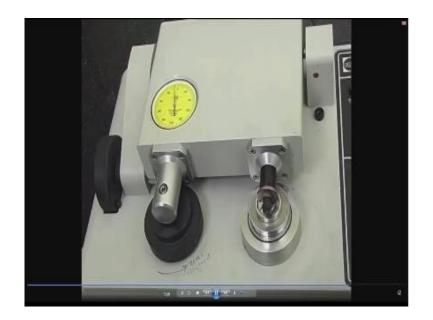
And then you have the grinding be and then the disc is kept on rotating in order to produce a dimple in the center of the 3 mm disc. And the thickness of the dimple is measured in this dial gauge. So typically you remove every micron thickness you will be able to monitor through this dial gauge and then you have the control over the RPM of this the disc.
