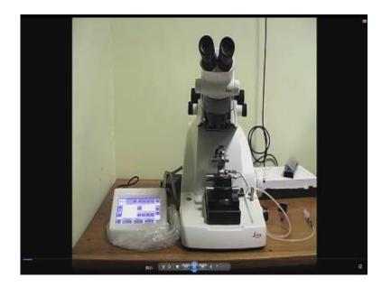
This is how the equipment would look like this is a ultra microtome it is very, very useful equipment for a polymeric sections preparing a polymeric thin sections again you have the stereomicroscope on this top and thi.
