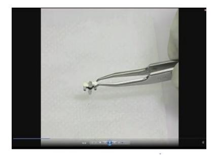
So the do post assembly is taken with the sample mounted on the clip now we will see how we can load this into the iron Miller.
