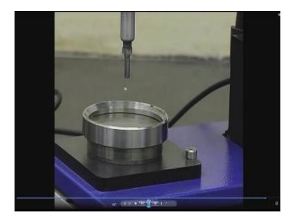
So that is the basic function and then you have the you have the facility to you know reduce or increase the frequency and this is the stage you can just move up and down and you can see that tool very closely so and here again you have the dial gauge you can prepare a samples with thickness to few microns.
