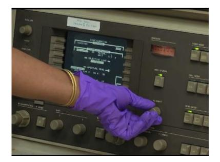
So what I am doing is I am heating the filamentous II there is just I am heating the filament you have to wait for until it is get a maximum electrons oh okay then from here you see here so many knobs are there so this is for magnification knob you can in this at cm tall microscope we can go
