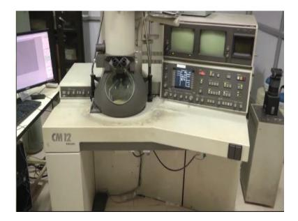
let us hear what you are seeing is a 120kv transmission electron microscope in the transmission electron microscope so we are using an electron beam to form the image because of the shorter wavelength nature of the electrons you are getting a high resolution in this transmission electron
