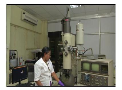
So from my anode it has to pass through the column to the bottom of the column okay so for that this electron should be were oscillated with a high speed because the electrons are pausing through the column in the column is under very high back up otherwise it will interact with the air molecule there should be a scattering effect to avoid that the whole column is under high ultra-high vacuum.
