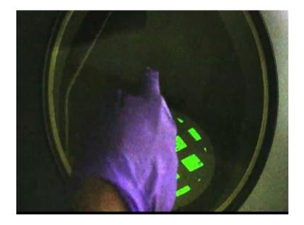
We have to wait for some time to get the filament heat what you are seeing is the image of your specimen so this is the folder sample say I have mentioned in cm12 there is a copper mesh on that there is a fine coating of a carbon film that is a few nano meter thickness on the carbon film
