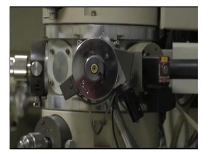
So if you see this is the specimen holder because the electrons is passing through the specimen your specimen thickness is very important you have to use a ultra-thin specimen okay so for the different methods are there to prepare the specimen so your specimen should not exceed 100 to 150 nano meter thickness other ways the electron will stop here itself okay to avoid that you have to make the specimen to 100 to 150 nanometer thickness by different methods for a
