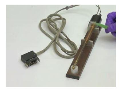
by using this holder you can heat the specimen inside the microscope you can continuously observe what is the heat treatment effect in this is a training holder you can give this you can strain the sample inside the microscope okay well observe a observing you can strain the sample and see the effect of that straining so we have two screws are there you loosen the screw and then you have to put the specimen here and then you can proceed.
