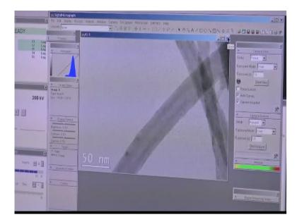
But further reduces resolution your this distance is 200 nanometer you will see the increasing the resolution this is 50nanometer okay we'll see this, this is a carbon nano tube and then when I am going further to that you see that this is a 5 nanometer image see here this is a fine animated image what you are seeing is a lattice fringes okay.
