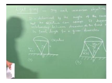
So I am kind of written a definition for the light grass of an objective lens it is determined by the angle of tone of phrase. That the objective can accept and it also depends on, depends on the relationship, between diameter of the front objective and, and its focal length for a given
