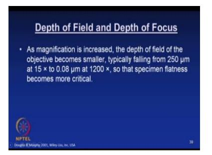
So now so this is the same thing as the magnification is increased the depth of field of the objective becomes smaller and typically falling from 250micrometer at 15 X to 0.08 micrometer at 12, 000 X it is a kind of range the specimen flatness becomes more critical so that is why you see that a very you know shallow depth of field once you cross this range.
