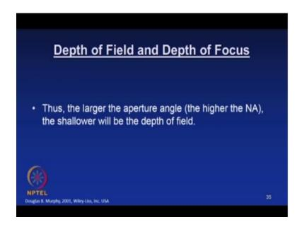
So that is the another aspect of the field of view let us now look at the come back to this depth of field and depth of focus, so the larger the aperture angle that means the higher the numerical shallower will be the depth of field and you can see this example a photograph
