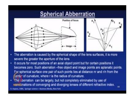
So we will see one by one and we will try to understand what are these defect really means first look at look at the spherical aberration look at this schematic what do we see we see that the rays which are coming close to the optic axis are focused the farthest and the rays which are passing through the periphery of the lens are focused in the nearest and the rays which are passing through in between these two are focused between this two points.
