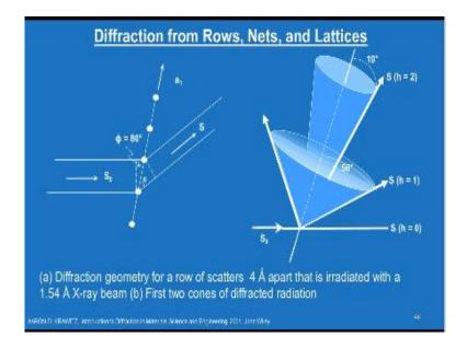
To look at the effect of the angle similar schematic where the incident angle is about 80 and then let us assume that the defection geometry for a row of scatter this is a row of scattering row of scatter is for angstrom that is irradiated with the 1.5 for angstrom x-ray beam so now you see that the value for  $\lambda$  is equal to I mean  $\theta$  is equal to a t 56 and 19 corresponding to H is equal to 0 h is equal to 1 and h is equal to 2 and so on.
