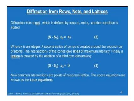
Now we will move on to the two dimension so diffraction from a net that means two dimension which defined by rows a1 and a2 another condition is added to the previous condition that is the  $s-s^0$ .a2 that is a path difference is also should also be equivalent to multiple I mean multiple of integral multiple of a  $\lambda k\lambda$  where k is an integer a second series of cones is created around the second row of atoms the intersections of the cones give lines of maximum intensity.
