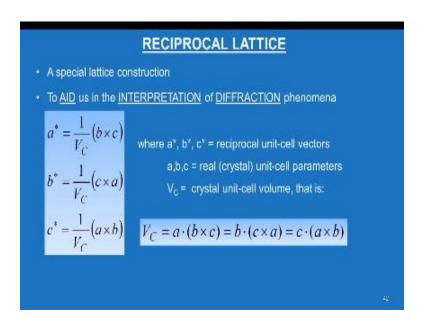
And excuse me what is reciprocal lattice, it is a special lattice construction to aid us in interpretation of the diffraction phenomena so this is the fundamental aspect of it and how this lattice parameters are reciprocal unit vectors are defined which is  $a^* = 1/V_c$  (b x c),  $b^* = 1/V_c$  (c x a) and  $c^* = 1/V_c$  (a x b) where  $a^*$  b\* and  $c^*$  they are all reciprocal unit cell vectors where ABC
