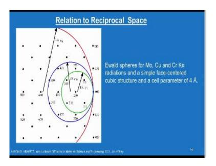
Where the evolve sphere for molybdenum copper and chromium k alpha radiations in analyzing the simple face centered cubic structure with the cell parameter for angstrom, suppose if you use one of this radiation for example let us use a chromium radiation so which is  $1/\lambda$  of chromium which forms the evolve sphere around these lattice points I mean reciprocal lattice points which
