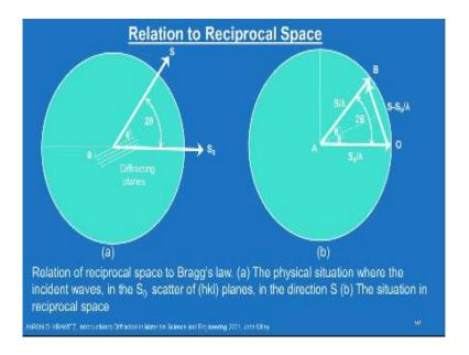
So what it says is this is the diffraction vector s which is nothing but R\* hkl in a reciprocal space so whenever this point hits on the surface of this sphere then the diffraction condition is satisfied and that is what is stated here.
