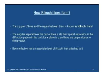
So the plus or minus G pair of lines and the region between them is known as Kikuchi band the angular separation of the pair of lines is  $2\theta$ . They are spatial separation in the diffraction pattern in the back focal plane is G and the lines are perpendicular to the G vector. Each reflection has an associated pair of Kikuchi lines attached to it.
