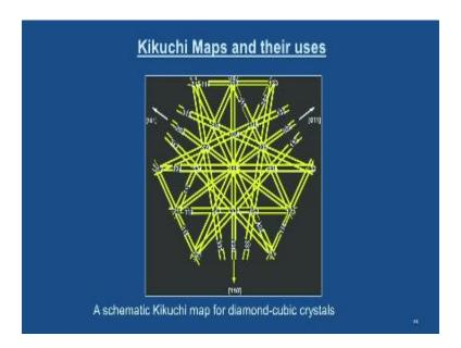
So this is the typical schematic of Kikuchi map for a diamond cubic crystal. So we will just see that some of the applications of this you can as I mentioned that you can map the grain orientations and orientation mapping and then you can identify the faces and you can quantify all the micro structural parameters. We will just show you some glimpses of all this if not in detail and the Kikuchi lines.
