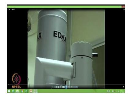
So what you are now seeing on the screen is in a scanning electron microscope I am going to explain to you in detail put all these features and this is how the equipment appears from the front side and this is the specimen chamber we are going to open this and then tell you what it can be so you can have a closer look this microscope is having at tungsten emission possibly a tungsten filament.
