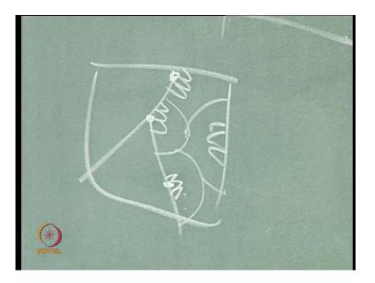
So, if you imagine that in one grain if you have different nucleating sides here. So, each of them will have a combination of a cup we call it as a couple ferrite cementite or cementite ferrite. So, once you have a cementite obviously, you will have ferrite on both
