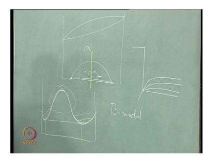
Let us now try to draw, the free energy curve at this temperature for this, if I draw the free energy curve, the free energy curve actually looks like this, am I right because when do you get a miscibility gap, when the delta h is positive. Whenever, the delta h is positive and that is higher than the t delta s mixing term, then you will see the free energy curve will have this kind of a shape.
