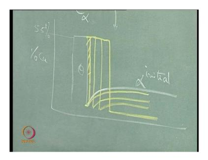
And as a result, now the theta grows by a small distance, but in the whole process, because the whole precipitation is happening at a fixed temperature, this value will never change, because this value is coming from the free energy diagram. And in the free energy diagram, the free energy diagrams are always drawn at a fixed temperature, at a fixed temperature, the composition of alpha in equilibrium with theta is fixed.
