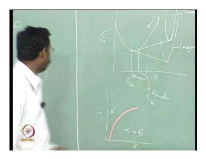
And we are talking about the starting composition alloy composition is somewhere here, that is the alloy composition with which you have started, which will be a two phase mixture and what we are talking about is a equilibrium composition of alpha. That means, if you look at the phase diagram, this is let us say alpha plus theta here, and this is alpha.
