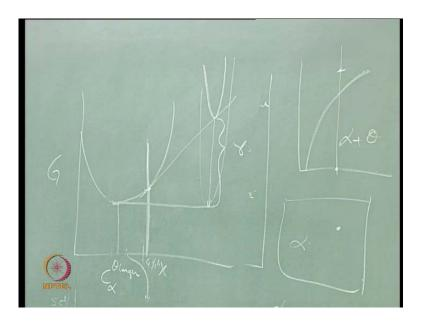
So, so the point is, if I look at let us not talk about all this, imagine I have started with an alpha of certain composition, this is a 4 percent copper, I started with this alloy and I am holding this alloy at some temperature. I am holding this alloy which is solutionized brought to this temperature quenched, and I am holding at that temperature, at that temperature is alpha stable, it is not stable.
