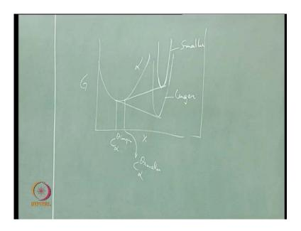
And if that is the case, if you draw that G h diagram, let us say this is the free energy composition diagram, this is of alpha, and this is let us say theta phase with a larger particles and theta phase with a smaller particle. This is you can call it as a smaller particle, this is a larger particle. So, a smaller particle will always have a higher free energy, when compared to the larger particles.
