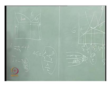
For example, if you take a phase diagram something like this, you take a eutectic composition. And, the moment you come below the melting point, below the eutectic temperature, bring this liquid, hold it at this temperature. What should happen?
