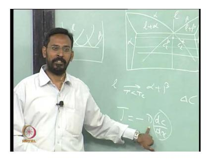
So, if I want to know what is the composition of liquid in equilibrium with alpha and liquid in equilibrium beta at that temperature, the only way I can find out is by extrapolating the two liquidus. So, if I extrapolate the two liquidus, I get this. And, this composition is nothing but C l what? Alpha. This is nothing but C l beta. And, the difference between these two is actually the driving force for the growth of eutectic. If
