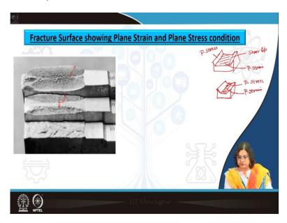
And if we try to see how the fracture surface looks like, we can see here that in case we have a thick component something like this, where we are getting the plane strain condition in the interior which is giving us a flat fracture surface as well as shear lip on the edges in which it is deviating to  $45^{\circ}$ .
