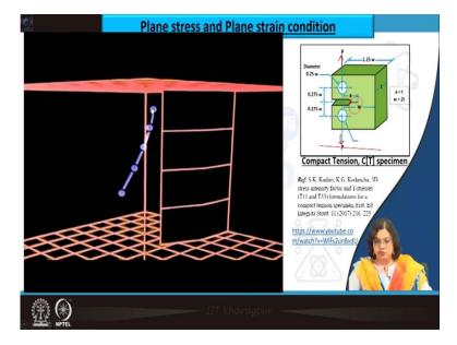
To obtain similar kind of values, if we are shifting the point upward, we need to shift it towards the crack also, to maintain this plane strain condition. And eventually, it has to be very very near to the crack tip to achieve this plane strain condition.
