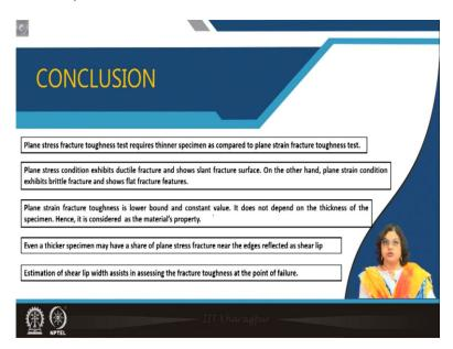
So, with this let us conclude this lecture what we have seen in this lecture is that the plane stress fracture toughness test requires a thinner specimen. On the other hand, plane strain fracture toughness, if we want to do we need a thicker specimen. Plane stress condition exhibits typically ductile fracture and that leads to a slant fracture surface.
