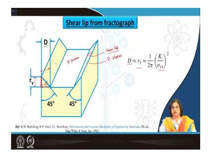
So, based on this, we actually can use this for the practical estimation of the K value or the fracture toughness values or the stress intensity factor value at that point of fracture just from this shear lip or from the fractograph itself. So, let us see how this can be done. So, this is a schematic of a fracture surface as we have seen.
