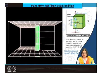
And that leads to a plane strain in the middle, but plane stress near to the surface for a very thick component.
