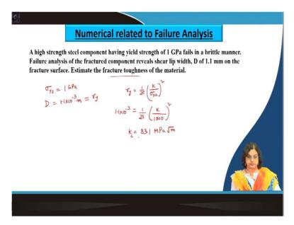
So, based on this there is a simple numerical to solve this and and to also appreciate that how fractographs and the information as well as the understanding can be used to pursue the failure analysis. So, it says high strength steel component which is having an yield strength of 1 GPa that fails in a brittle manner and failure analysis of the fractured component reveals shear lip width.
