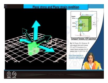
Now, when we are talking about the thin component, you see the plastic zone here is pretty big that is encompassing the entire thickness and we are applying the tensile stress along this direction which leads to a stress perpendicular to it, which however is 0.
