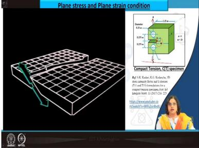
And then there is a shear stress also 45°. And accordingly the crack will move along the shear planes and that will lead to a slant fracture surface. So, that is what we essentially see in case of plane stress or plane strain condition.
