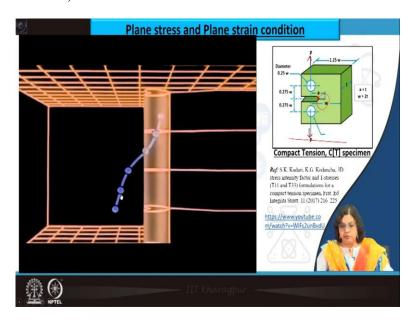
But, so far, we have not talked about the plastic zone and its influence. So, in this case in presence of this plastic zone, these points are actually moving near to the surface and near to the crack tip to achieve the plane strain condition. And eventually, it will be just embedded within the plastic zone itself, leading to the plane stress condition being active towards the surface.
