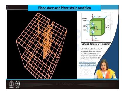
So, here is a video which explains how the plane strain and the plane stress mechanisms are active. So, this is particularly done on a compact tension specimen which is typically used for fracture toughness testing. So, this is three-dimensional specimen that you can look for. This one is quite thick here and when we are loading in along this direction, the crack which is perpendicular to this loading direction, expands along this direction.
