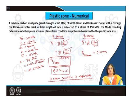
And to understand that we would like to solve a numerical to understand this concept further. So, it says a medium carbon steel plate with yield strength of 350 MPa and width of the plate being 80 cm and thickness being 1.5 mm. It has a through the thickness that means a center crack of total length 40 mm. And it is subjected to a stress of 150 MPa.
