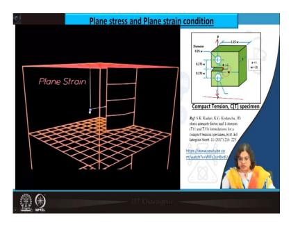
Now, plane strain fracture toughness of a material is varied for one material to another. When we are talking about a three-dimensional space, let us talk about a point which is at certain depth from the surface and at some distance from the crack tip. And it is in the plane strain condition because it is in the constrained stress.
