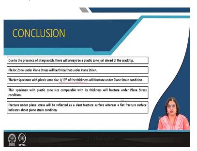
Based on this let us conclude today's lecture that what we have seen is that due to the presence of sharp notch there will always be a plastic zone ahead of the crack tip and this plastic zone under plane stress condition will be bigger and it is almost three times bigger than that under plane strain condition. Now, thicker specimen will have this plastic zone size, which is
