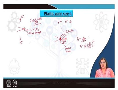
So, moving on to the very first concept about the plastic zone size. So, we have seen that the linear elastic fracture mechanics is based on the basic assumption that cracks are inherent in the material. So, in case there is a component with a crack in it and we are applying stress like this, tensile stress in the mode 1 condition, which is perpendicular to the growth of the crack, then we have also seen that at the tip of the crack, we are getting a maximized stress and that
