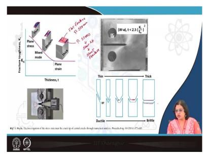
So, this is how it looks like in case of thin specimen. We are seeing that there is a pronounced shear lip, pronounced plastic zone which you can see in this blue zone. In case of mixed mode this shear lip width is decreasing and the shear of this flat fracture is keep on increasing. On
