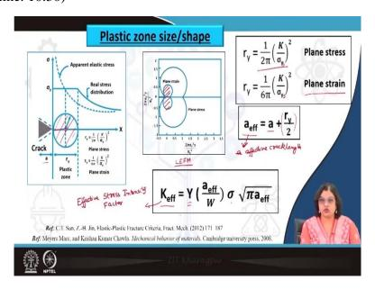
So, as I mentioned that this is the zone for the plastic deformation to occur and the stress value is continuously decreasing and that leads to a condition similar to this which are the
