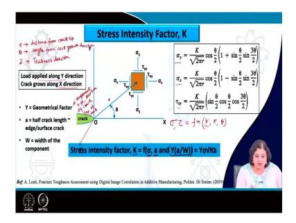
So, this is the situation where we have the x and the y axis and the z axis also along this. So, along the y axis load is being applied and crack grows along the x-direction, whereas z represents the direction of the thickness, so, let us say this as the thickness direction. Now, if there is a crack here and we are applying stresses along the y-direction, we want to figure out that what would be the stress at any point away from the crack tip.
