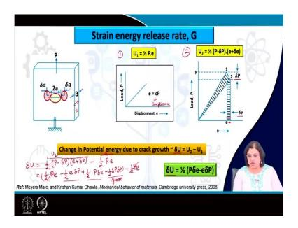
So, coming to the strain energy release rate, we have seen in the last lecture that strain energy release rate is nothing, but the potential energy that is stored in our system or in a component as the crack grows, whatever energy is being released, that is considered as the strain energy release rate and that is relevant for determining the fracture strength of a material as per the
