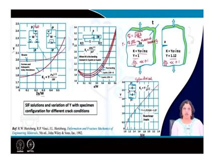
So, this is how Y varies as we are changing this parameter 2a / W, 2a is the total crack length and W is the width of the component. So, it has been seen as well as experimentally validated these are some experimental results that are being shown here that if the position of the crack varies and as we are changing this to a / W, you can see that this parameter Y is increasing.
