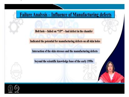
Apart from that there is something else also that were had made a significant impact on the failure analysis. What they found is that the bolt hole failed on this aircraft and that had a defect in the chamfer. So, this indicated the potential for manufacturing defects on all the skin holes.
