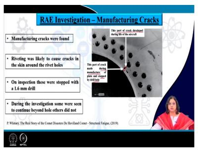
And what they could understood from the detailed study is that, so some part of the hole that has been punched that lead to formation of a crack during the manufacturing process itself and that could have been stopped by drilling a hole. However, you can see that this part of the crack developed during the life of the aircraft.
