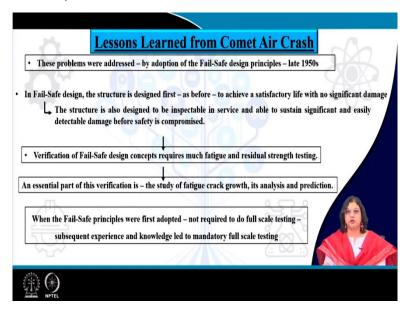
So, these problems were addressed by the adoption of Fail-Safe design in the late 1950s, in Fail-Safe design the structure is designed first as the previous one and to achieve a satisfactory life with no significant damage.
