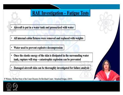
And the aircraft is also put in a water tank and pressurized with water, so another effort, this is the way by which the aircraft is put in a water tank and pressurized with water all the internal cabin fixtures were removed and replaced with weights and water is used to prevent the explosive decompression.
