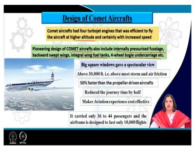
So, comet aircraft had four turbojet engines that was efficient to fly the aircraft at higher altitude and certainly with increased speed. So, that was the main key point for the comet aircraft that this one is the first one to use the turbojet engines that we use these days. So, you can see the engines here two on this side and two on the other side of the wing where there are the four turbo jet engines are located.
