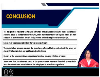
So, the conclusion of this lecture as follows, the design of de Haviland Comet was extremely innovative that accounted for faster and cheaper aviation. It had a number of new features, most importantly the turbo-jet engines which are now accepted as part of modern aircraft design.
