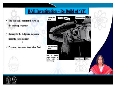
So, all the structures, all the parts as recovered from the wreckage you can see that they have been arranged and the tail plane were separated early in the breakup sequence and this damage on the tail plane is by the pieces form and the cabin interior you can see the carpets also hanging here got stuck actually and the pressure cabin must have been failed first which is what we have noted from the video also.
