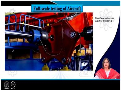
So, let us see here what I mean, you can see here that a full aircraft a total aircraft one is being tested for fatigue and all the parts, the wings and the fuselage and the engine parts and all the different parts are being tested in the service condition to understand whether it is capable of performing at those particular conditions and if it is so then for how long, for how many cycles or how many flights can be covered by this kind of aircraft.
