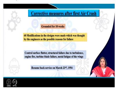
So, following that some corrective measures were taken. So, the aircraft companies were grounded for 10 weeks to do some detailed survey about what went wrong and they really did a detailed survey based on what could have been the possible reasons for the failure and they could come up with around 60 modifications in the designs which were implemented in the next level and then it has been used again.
