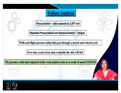
Now what could be the possible reason? Actually during the pressurization the cabin expands like a balloon of course it is a metal one so it will not expand like the rubber balloon but it still expands by about one eighth of an inch and of course during the depressurization so when the pressure is being removed, let us say during the landing or when it is at the lower amplitude, at that point it is this kind of expansion is coming back to the 0 level.
