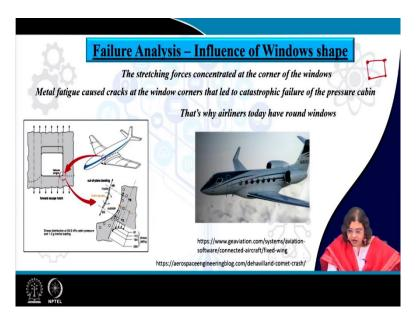
Now they have also realized that when such kind of experiments has been performed, the cracks has to initiate from some location and in most of the cases they have seen that the stretching forces concentrated at the corner of the windows.
