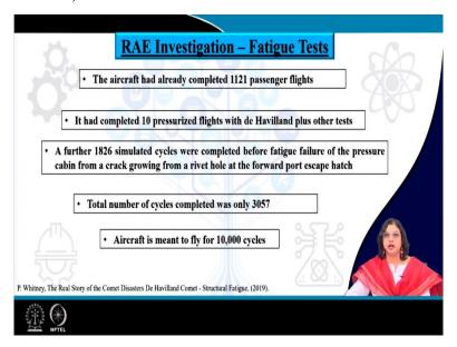
Now what they found is that, the initial known fact was that the aircraft had already completed 1121 passenger flights, the one which has been tested. It has also completed 10 pressurized flights with de Haviland plus other kind of tests initially. And during this kind of simulation
