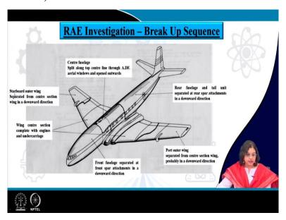
So, this is the sequence of the failure that has happened the centre fuselage. So, this part here with the top windows that split along the top centre line and the aerial windows had open outwards and then the starboard outer wing separated from the centre section wing in the downward direction and wing centre section complete with engines and undercarriage and the
