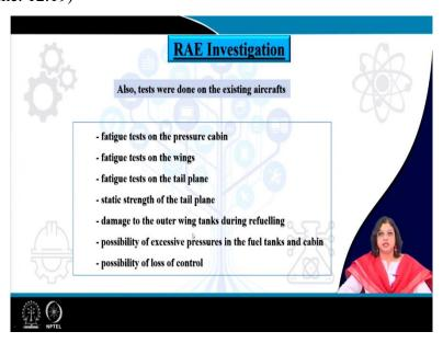
So, let us see what has been done. So, tests were done on the existing aircrafts one which are already there and which has not undergone any crash and for those fatigue tests were done on the pressure cabin, on the wings and as well as on the tail plane, static strength of the tail plane
