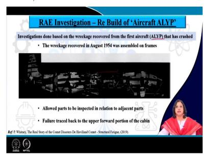
Now that was the investigation that was done based on the available aircraft through the lab scale experiments. On the other hand, investigations were also done based on the wreckage recovered from the first aircraft that has crashed. Now out of all the crashes this one for this particular one which was actually the first aircraft A-LYP for that major part of the wreckage could be recovered and that is the reason that they have performed a detailed analysis of what went wrong.
