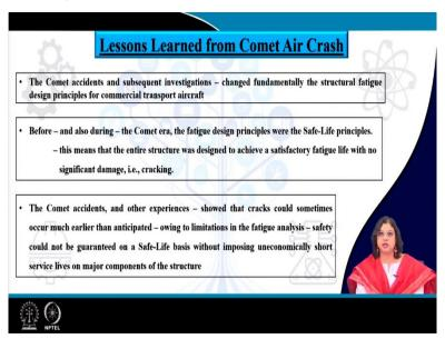
So, whatever lessons that has been learned from the comet air crash are the following, the comet accidents and subsequent investigations they have actually changed the fundamentally understanding of the structural fatigue design principles which are should be used for commercial transport aircraft.
