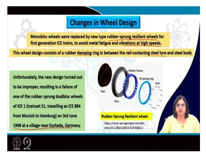
Now, what exactly is this new wheel design? To understand that, let us look into the picture how it looks different from the monoblock wheels. So typically, this new rubber sprung resilient wheels were used to avoid this vibrations at the high speeds. And this kind of wheel consists of a rubber damping ring in between the rail contacting steel tire and the steel body. You can see the rubber blocks here, which is actually helpful for avoiding the vibration.
