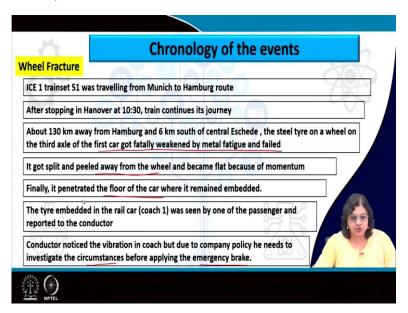
So, wheel fracture is one of the main incidents here. So initially, the trainset 51 was traveling from Munich to Hamburg route. And it after stopping at Hannover at around 10:30 in the morning. It continues its journey while at around 130 kilometers away from Hamburg, and 6 kilometers south of Central Eschede the steel tire on the wheel on the third axle of the first car got fatally weakened by the metal fatigue and failed.
