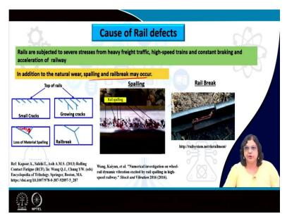
So, the same thing happened here also, along with that, there are some other reasons, which are typically found as the rail defects such as the rails are subjected to severe stresses from heavy freight traffic, high speed trains and constant braking and acceleration of railway. So, because of these fluctuations in the load levels also, along with the natural wear, spalling and rail break may occur.
