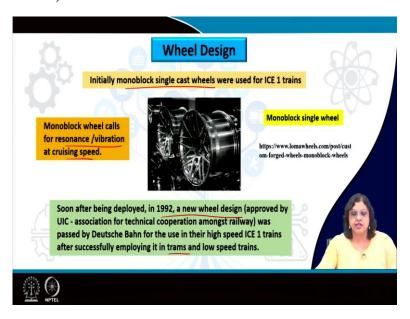
And typically, such kind of high-speed trains were initially using monoblock single cast wheels. Here is a picture of the monoblock wheel how it looks like. However, such kind of wheels often leads to the resonance or formation of some vibration at the cruising speed, and that often leads to some kind of turbulence and are not very much favored.
