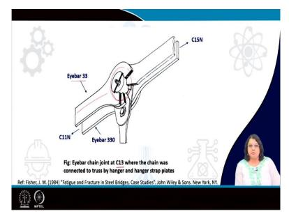
And this is what is known as an eyebar. So, you can see that there is one. So, this is one eyebar part of one eyebar which has a circular section followed by a certain length and then there is another eyebar which is connected to it through this pin. So, this is one particular section showing C13. So, all these eyebars are numbered and there are several hundreds of such eyebars in the entire bridge structure.
