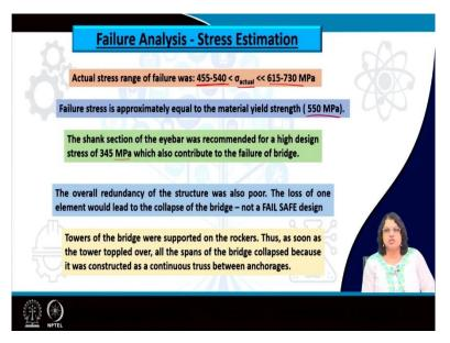
And this gives the actual stress range at the point of failure is lying between this 455 to 540 which is the lower bound and the upper limit is 615 to 730. It might have been within this 2
