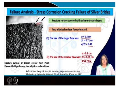
So, detailed fractographic analysis you can see that this is the fracture surface and then they have been pointed the location for 2 cracks here. The entire fracture surface has been noted to be covered with rust first of all and then the adherent oxide layers. And after removing those oxide layers and the rust it has been noted that there were 2 elliptical surface flaws as pointed here with the arrows.
