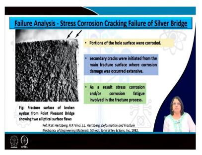
So, it was also realized that portion of the holes, you know the eyebar which is having the hole in it, that is seems to be corroded as well. So, secondary cracks were initiated from the main fracture surface where corrosion damage was occurred extensively. And as a result of this stress corrosion and corrosion fatigue gets involved and that might have led to the fracture surface. So, these are all the presumptions that has been taken at the point of the failure analysis.
