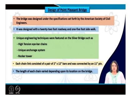
And the bridge was designed under the specification set forth by the American Society of Civil Engineers. So, it was designed with a 22 feet roadway and a 15 feet sidewalk. And the unique engineering technique were featured on the Silver Ridge such as it has very high tension eyebar chains that were used and unique anchorage system, rocker tower et cetera. All those things were once again considered as engineering favorable structures and are used in this bridge.
