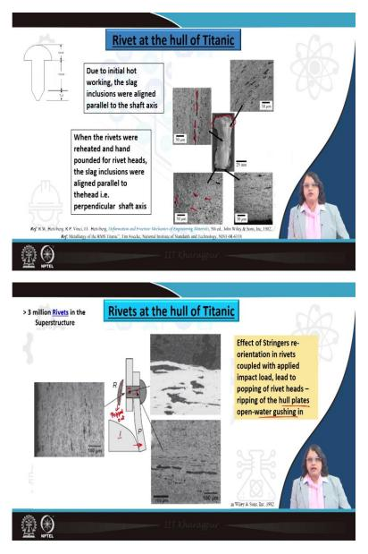
Now, what happens is when it hits the iceberg. So, this is the example how the inclusions are aligned along the shaft axis perpendicular to the head and along the head however, these are aligned perpendicular to the shaft axis. So, this is what we can understand from here. Now, this would not have been a problem this difference in the alignment of the stringers on the shaft or on the head would not have been a problem. In case there was no load applied, but,
