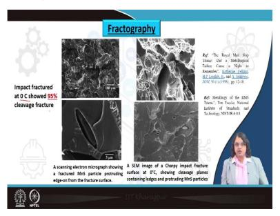
But in any case, we have seen for the Titanic that DBTT is quite low, when we have looked into the fractography in details, the impact tested carried out at 0 °C showed 95 % cleavage fracture. Once again signature for brittle failure and that means that it has already undergone to brittle nature at that temperature of 0 °C itself.
